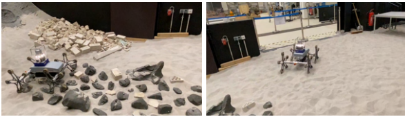
Figure 9: Field test setup for terrain classification.
